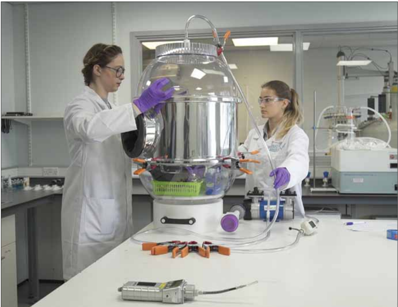
The BSTL environmental test chamber as used to replicate the NIOSH test protocol for assessment of CSTD systems.
