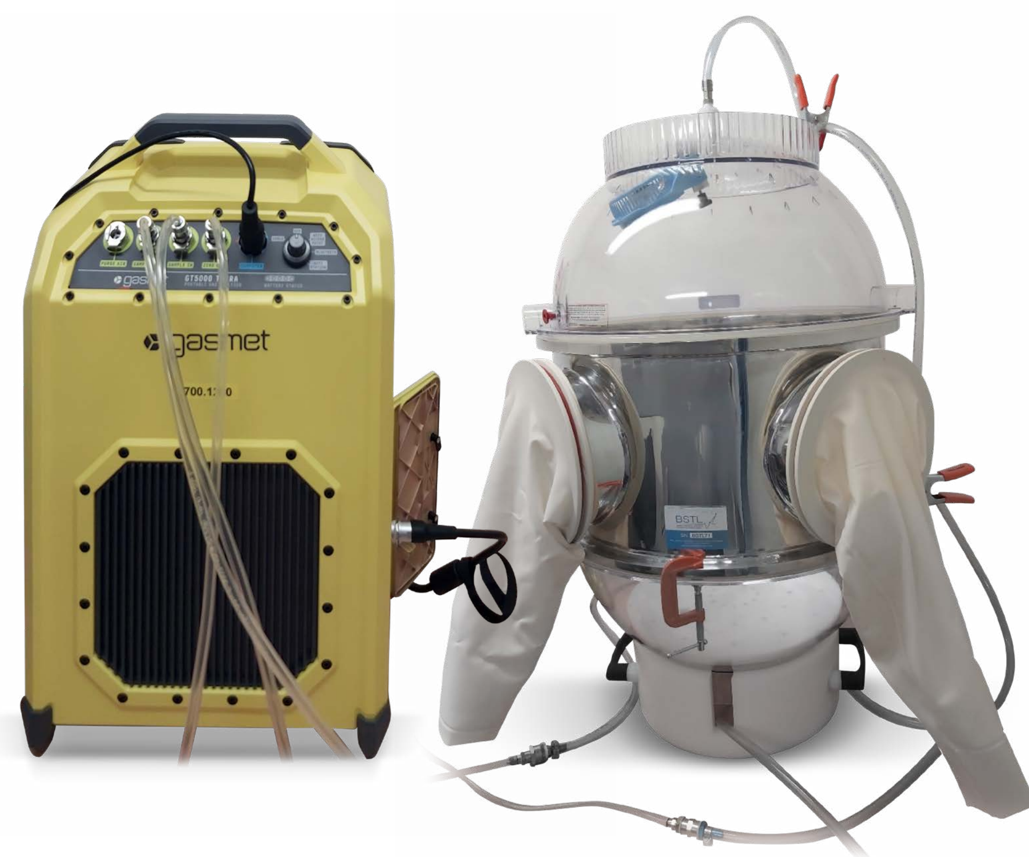
Figure 2 Left: Gasmet GT5000 Terra gas analyzer for online ethanol vapor quantification. Right: sealed glove-box chamber inside which tested CSTD products can be manipulated for vapor containment testing in a closed environment.
