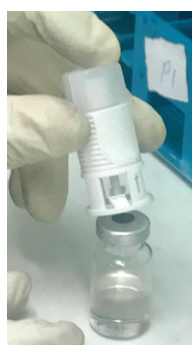
Figure 1: Assembly of a Vial Adaptor to vial
