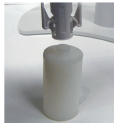
Figure 2: Septa extraction using distilled water in a designated recovery fixture
